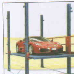
Floor to Floor Lift
